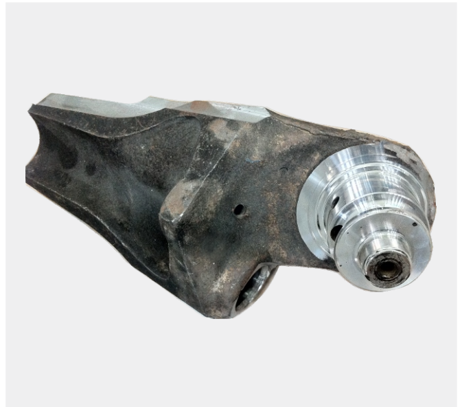
牙爪外圆车削 PCBN external turning for tricone bit
