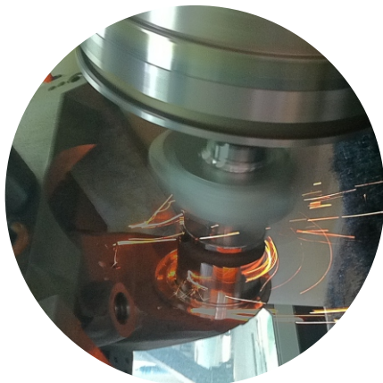
牙爪外圆铣削 PCBN external milling for tricone bit
