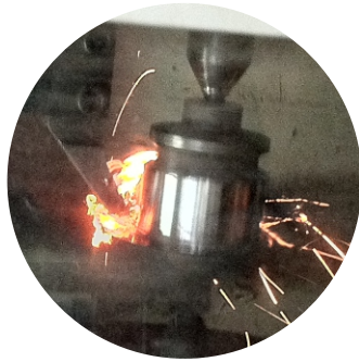
牙爪外圆车削 PCBN external turning for tricone bit
